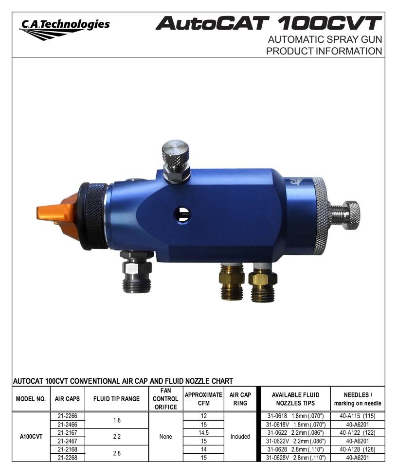
Actual fluid nozzle and air cap combinations are determined by application Fluid nozzles ending in "V" are carbide fluid tips
